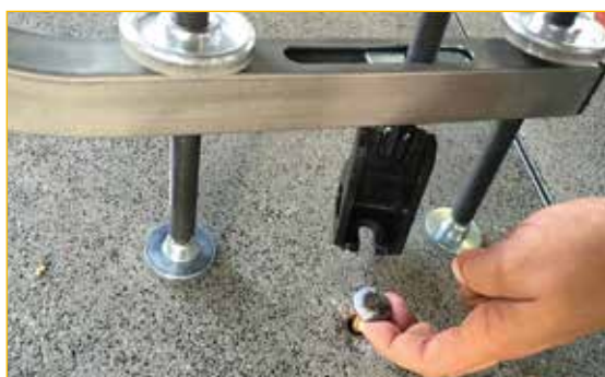
Central tie rod with rotating and sliding hook. In central picture visible female coupling.
