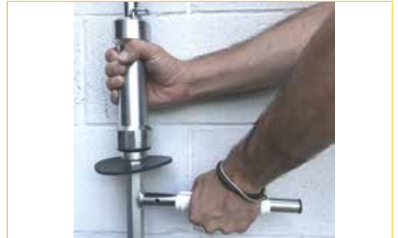
Safety pin when hammer is not in use.
