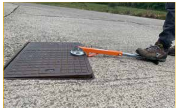
Cover release with central pin
