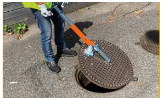
Use 3: Opening with horizontally extended handle bar.
