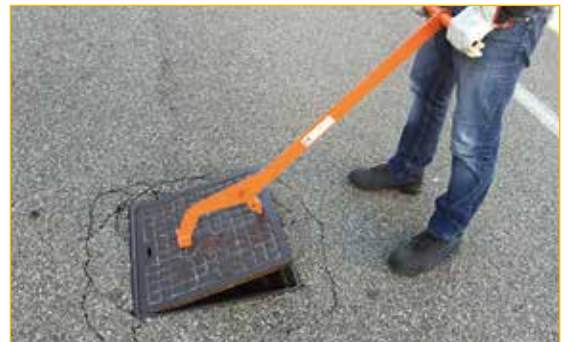
In the opening operation, the length of the lever limits the operator effort.
