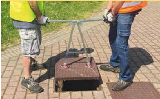
Lifting power up to Kg.460.
