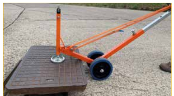
Lifting with wheeled levers APS80 or APS90
