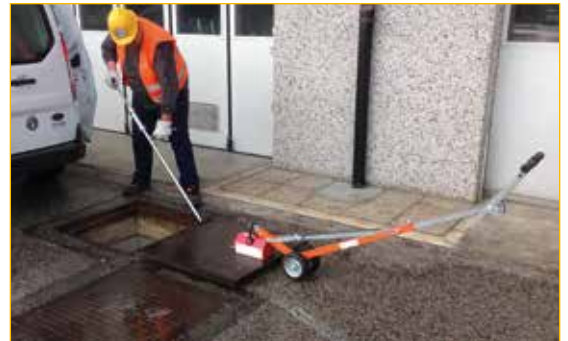
MZ120 particular shape allows you to unlock the safety lock of the lids and, subsequently, to be used as a lifting lever.
