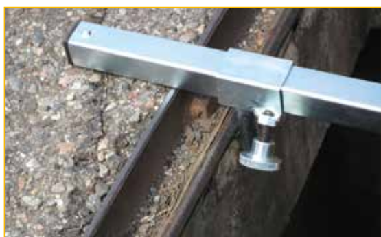
Sliding and adjustable struts at the tip of the arms to keep the cross in the correct position.
