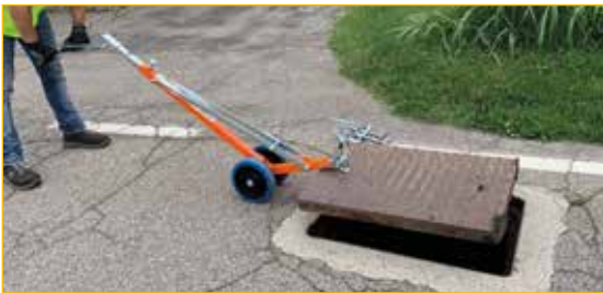
Use 3: mechanical opening with locking clamps.
