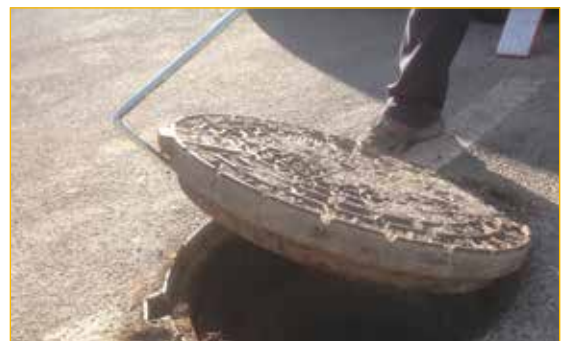
Built in tempered 38NCD4 steel with galvanized anti rust finish which makes the LB7 a resistant and robust tool.
