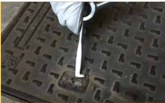
Configuration 2: L - shaped end for scraping in the inside of the slot and release the rotation for opening the lid.
