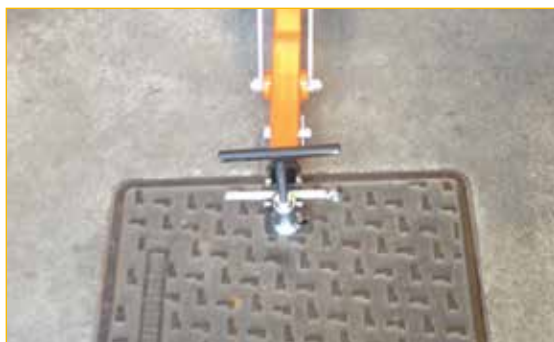
Phase 2: engagement of the lever in the clamp.
