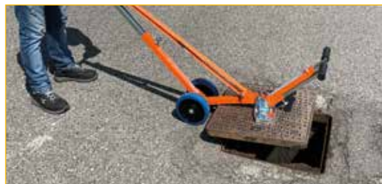
Use 1: opening with magnetic CL9 - CL10 - CL11.
