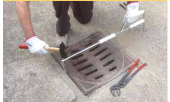
The beaks can also be used in the operations of scraping the frame of the lid.
