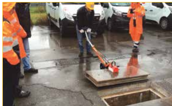
Use 1: necessary use in the presence of manhole covers excessively heavy or worn out.
