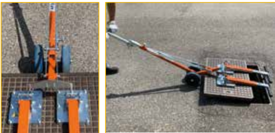
Use 2: opening with two CL10 in parallel joined with connecting "bridge" on heavy lid.
